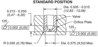
Flow is regulated from a hydraulic cylinder or motor, to the control valve
